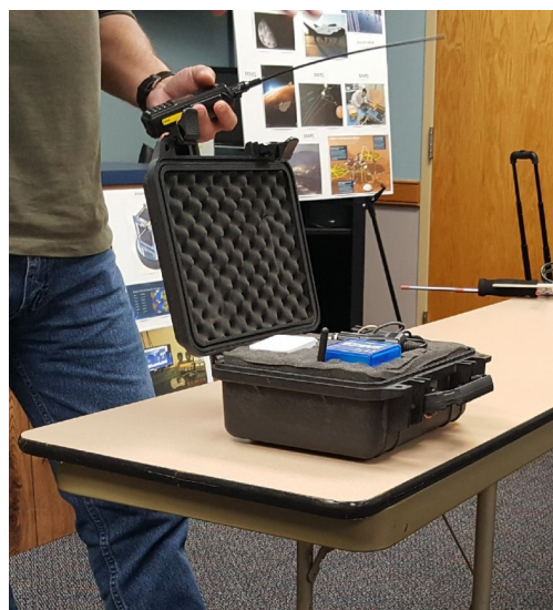
Carlos Arzuagas W9FE demonstrated his DMR HT along with his Hot Spot which allows him to connect to the internet when a digital repeater is not within range. His hot spot go kit allows him to use his DMR HT to connect with talk groups almost anywhere he goes. He has it enclosed in a protective case
